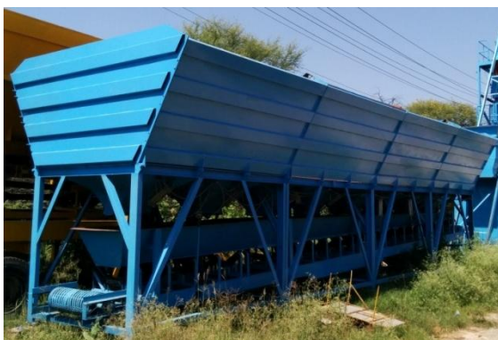
A FOUR STORAGE HOPPER AGGREGATE SUPPLY SYSTEM WITH 15 M 3 HOPPERS
